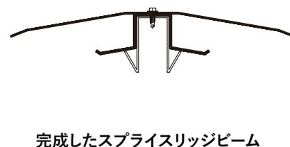
**PRE-ASSEMBLY OF SPLICED RIDGE BEAM**
