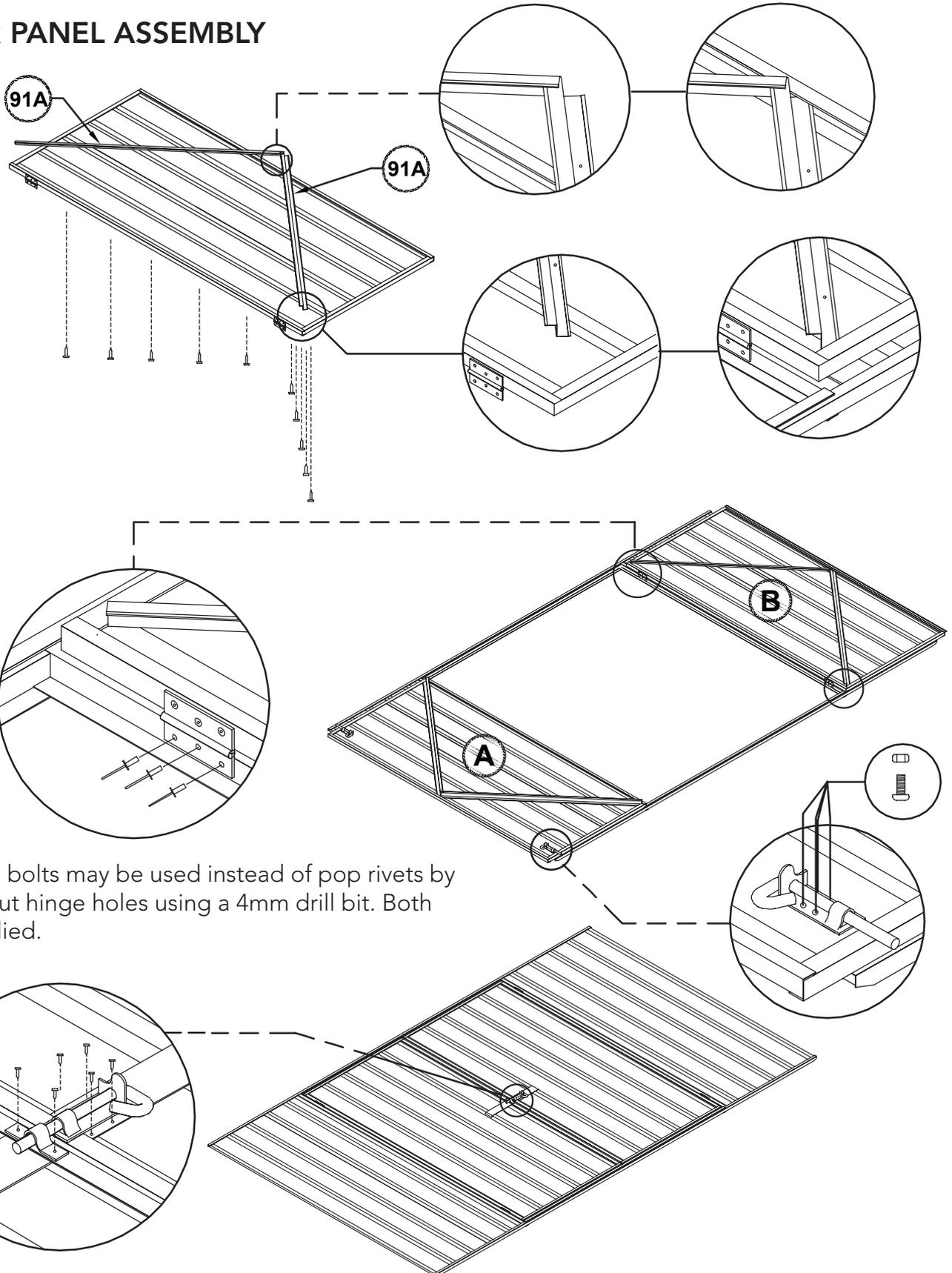
Nuts and bolts may be used instead of pop rivets by drilling out hinge holes using a 4mm drill bit. Both are supplied.
