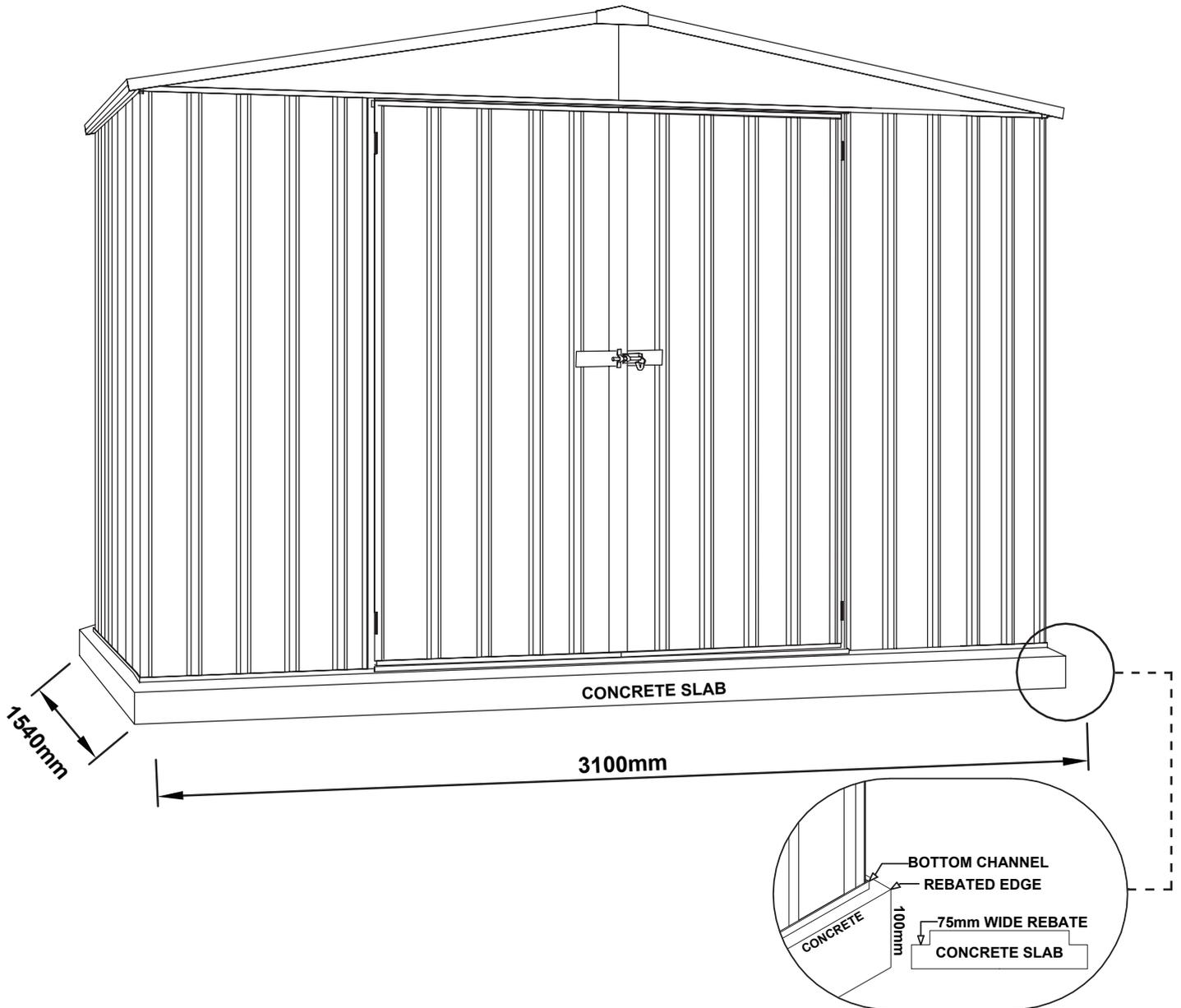
When laying concrete slab, ensure there is a rebated edge 25mm deep around the perimeter. This will help water egress from the base of the shed.
