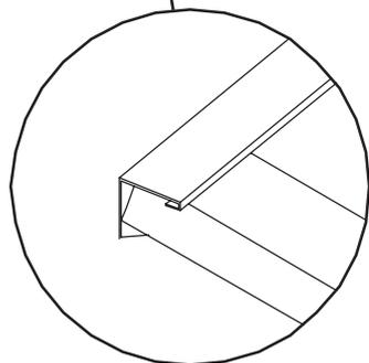
The notched end of the channels are to be positioned to the sides of the panel
