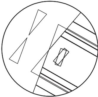
NOTE: Trim the tips of the centre sheets with tinsnips to allow channels to fit hard up to the edge of the sheet before attaching channels.
