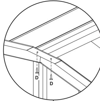
Drill new holes in the ridge beam (3mm bit) through the peak brace and fix with a FAST001 after the roof panel is inserted
