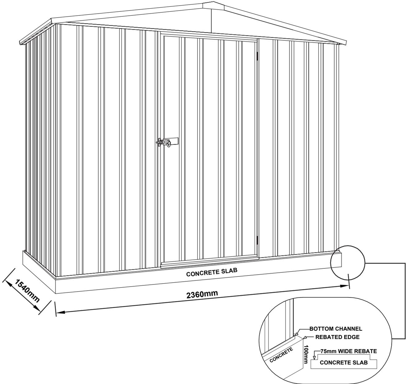
When laying concrete slab, ensure there is a rebated edge 25mm deep around the perimeter. This will help water egress from the base of the shed.
