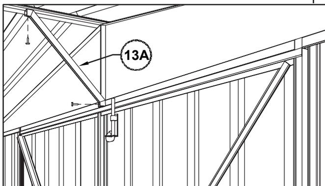
After attaching both roof panels to walls as shown above, fit one regent brace to the ridge beam and front wall as shown. You will have to remove and replace existing screws at fixing locations.
