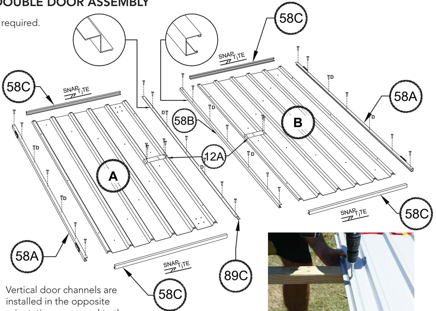
Vertical door channels are installed in the opposite orientation compared to the horizontal door channels.
