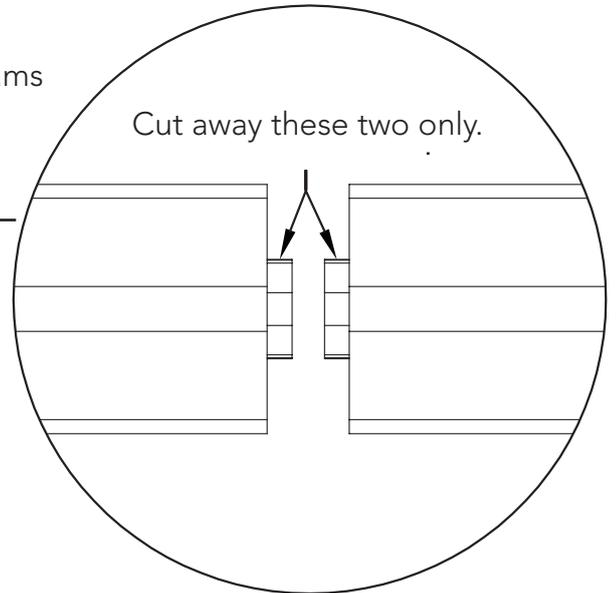
Using a hacksaw, remove one protruding section of each ridge beam, this will allow the sections to butt up neatly to each other.
