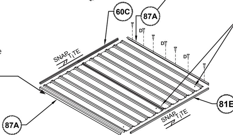
Fit 81E to edge of sheet with pre-punched holes.
