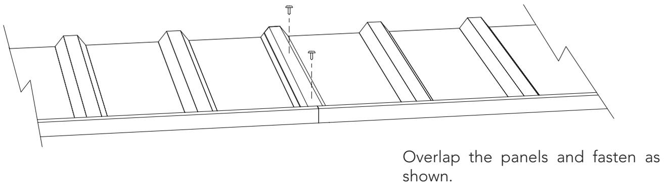
Refer to the panel construction section of this instruction set for further details and ensure that the assembled panels are not joined together with pre-punched holes incorrectly positioned.
