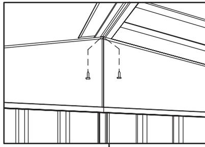
Secure ridge beam to gable sections with two screws at each end. Secure each roof panel with one screw in each corner only at this stage
