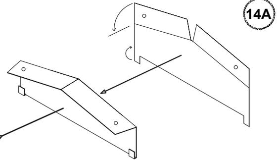
Bend the top and bottom flanges as shown, then hook the bottom flanges under the top channel and screw top to the ridge beam with two screws.
