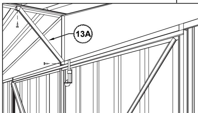
After attaching both roof panels to walls as shown above, fit one regent brace to the ridge beam and front wall as shown. You will have to remove and replace existing screws at fixing locations. Repeat this procedure for the rear wall regent brace
