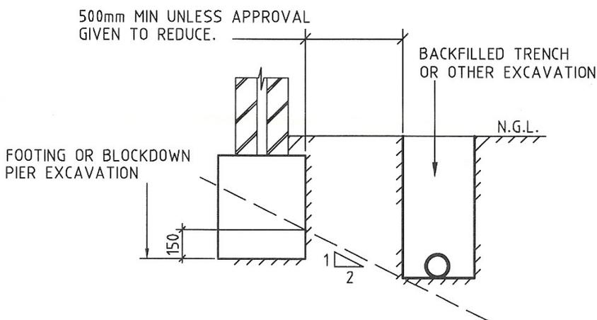
The contractor shall undertake investigatory localised excavations near existing footings to ascertain their depth prior to excavating adjacent to them. It is noted that excavating to a depth below that indicated above shall not be undertaken without the written approval from the engineer.
