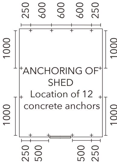
Each anchor consists of one nut, bolt, M10 dynabolt and steel angle.
