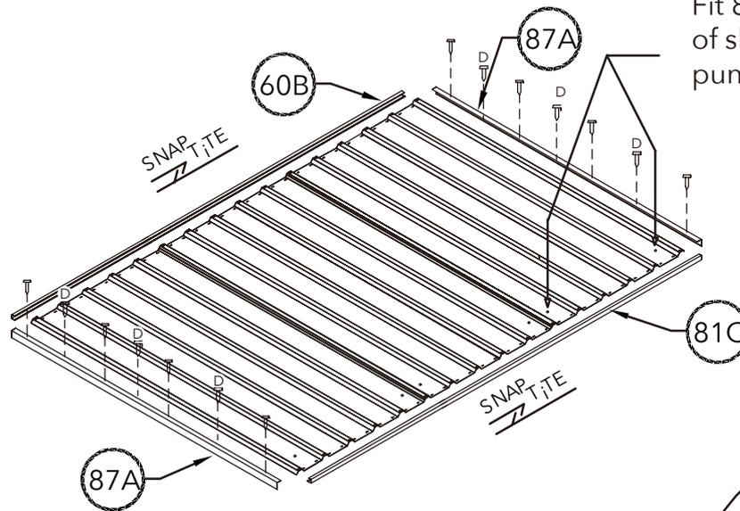
Fit 81C to edge of sheet with pre-punched holes.
