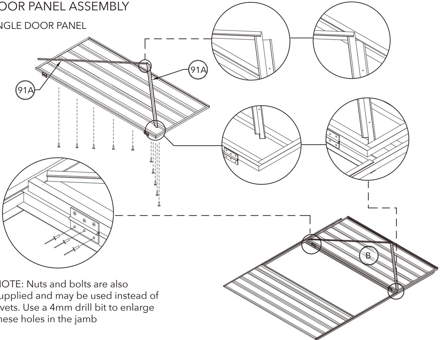
NOTE: Nuts and bolts are also supplied and may be used instead of rivets. Use a 4mm drill bit to enlarge these holes in the jamb
