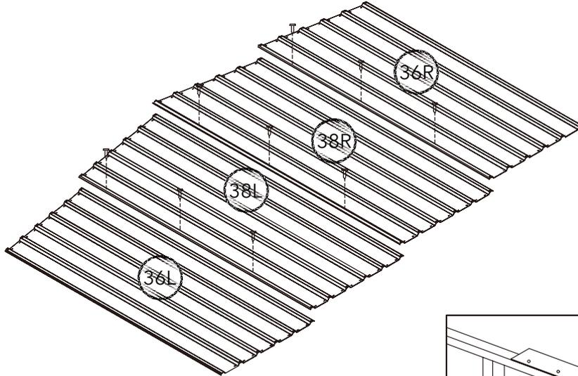
Trim the tip of each sheet or bend out of the way to allow channels to fit hard up to the edge of the sheet.
