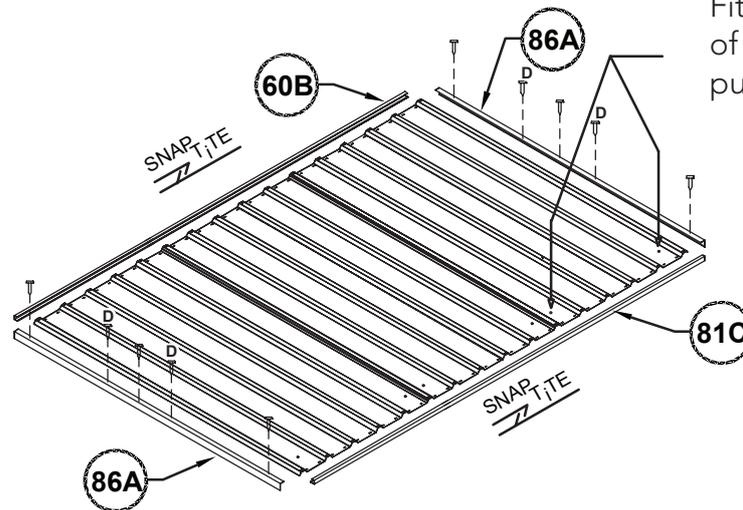
Fit 81C to edge of sheet with pre-punched holes.
