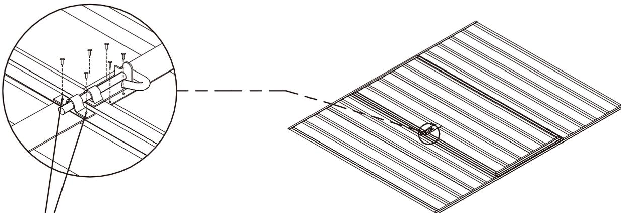
NOTE: The two holes required to connect the padbolt for each door have not been pre-punched, to allow for proper alignment. position each hasp centrally over the padbolt shaft, and drill 3mm holes and secure with screws
