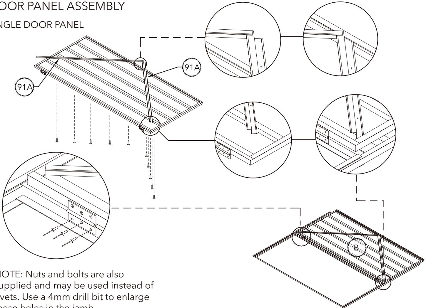
NOTE: Nuts and bolts are also supplied and may be used instead of rivets. Use a 4mm drill bit to enlarge these holes in the jamb
