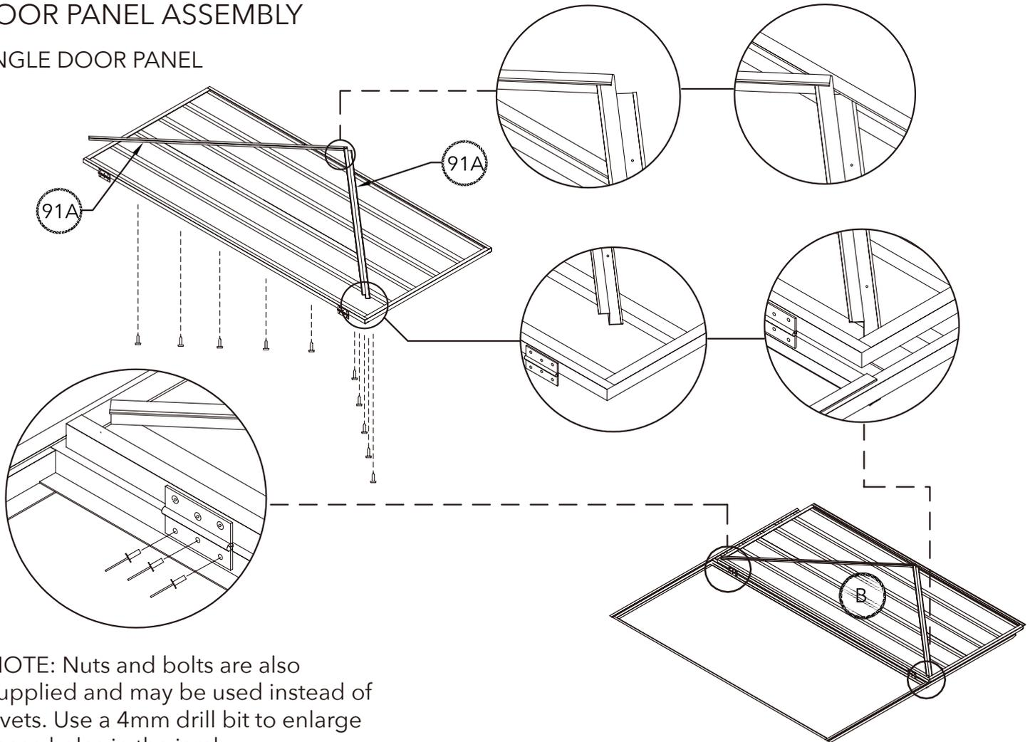
NOTE: Nuts and bolts are also supplied and may be used instead of rivets. Use a 4mm drill bit to enlarge these holes in the jamb
