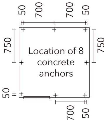
Each anchor consists of one nut, bolt, M10 dynabolt and steel angle.
