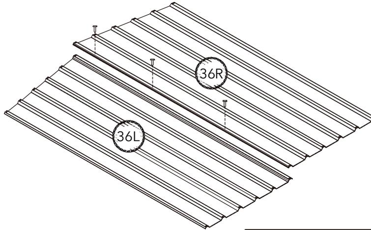
Trim the tip of each sheet or bend out of the way to allow channels to fit hard up to the edge of the sheet.
