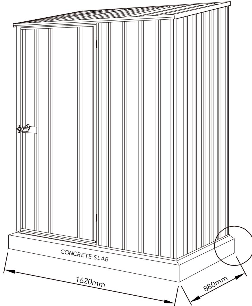
When laying concrete slab, ensure there is a rebated edge 25mm deep around the perimeter. This will help water egress from the base of the shed.
