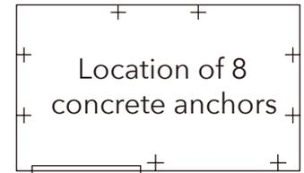
Each anchor consists of one nut, bolt, M10 dynabolt and steel angle.
