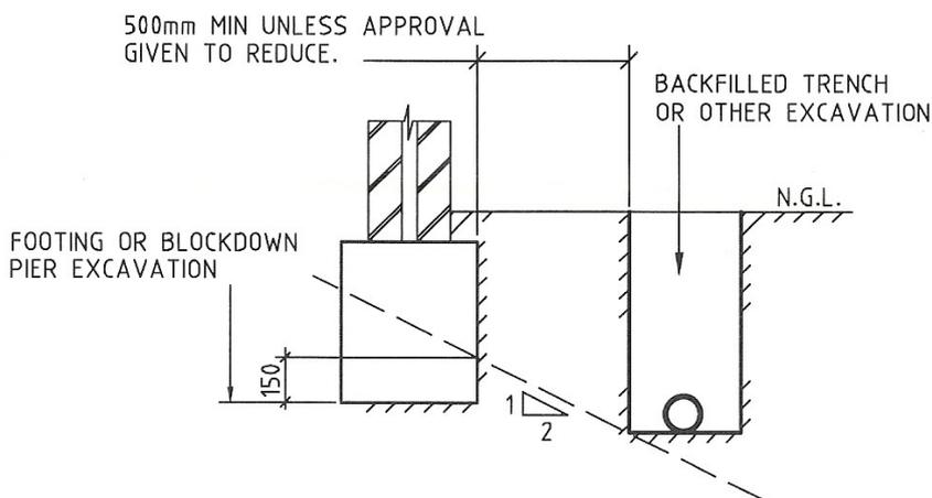
The contractor shall undertake investigatory localised excavations near existing footings to ascertain their depth prior to excavating adjacent to them. It is noted that excavating to a depth below that indicated above shall not be undertaken without the written approval from the engineer.
